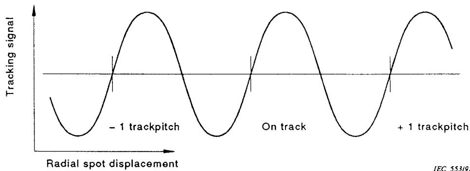
Typical shape of the error signal for tracking versus radial spot position.
